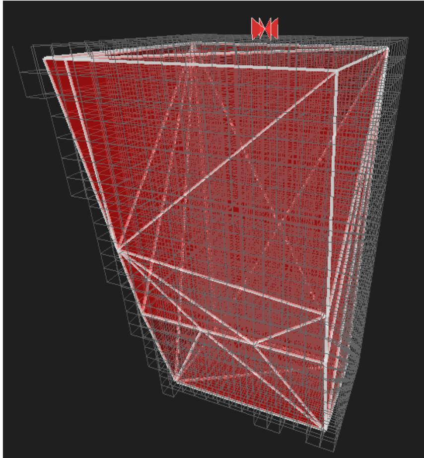
Within the main menu you can adjust the fill point position (reticulation discharge point), which is denoted by the red flag marker on top of the stope. Positioning of the fill point can be a crucial step in optimising your composite pour, particularly when working with steep beach slope angles and long/wide stopes.
